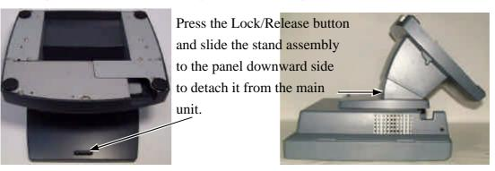
In order to properly install the TP-6000 terminal, all cables must be routed through its base. Therefore, please press the lock/release button at the rear side to separate the main unit from the stand assembly.
